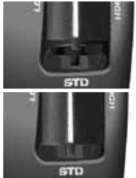
②Hold the special torque wrench in your right hand.(Attach the angle adjustment bit) and align the pawl on the angle adjustment bit with the indent on the angle adjustment unit and loosen the screw by turning the special torque wrench one or two rotations counter-clockwise.
