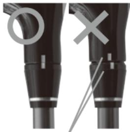
※Please take off the shaft from golf club if it does not turn smoothly. There is a possibility that screw is not engaged with grooves, or contamination such as sand, dirt and grass is in the groove. If you continue to turn it, it might cause damage and defect.
